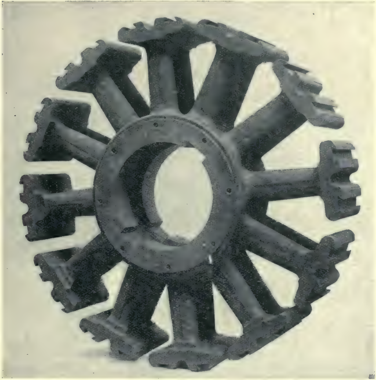
FIG. 57.—Photograph of Armature Spider of large Generator. Vickers, Sons & Maxim.
